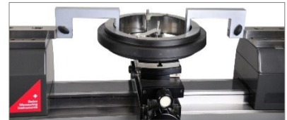
Checking of ring gauges from 12mm
