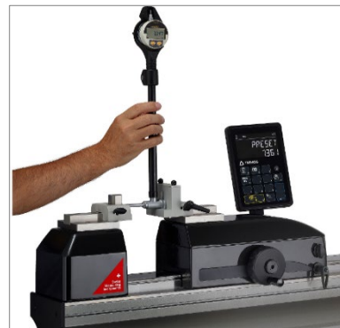
Setting manually of 2-point bore gauges (TA-SU-301, TEL5)
