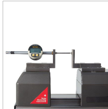
Checking of dial indicators and comparators (TEL 5CN)
