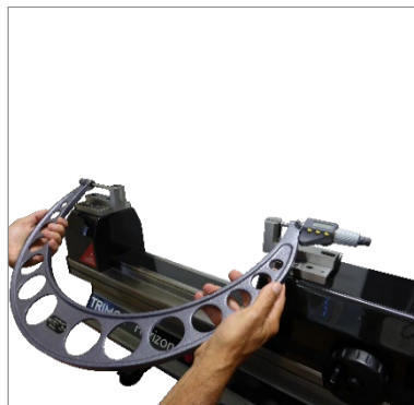
Manually checking of external micrometer (TEL5, TEL 11)
