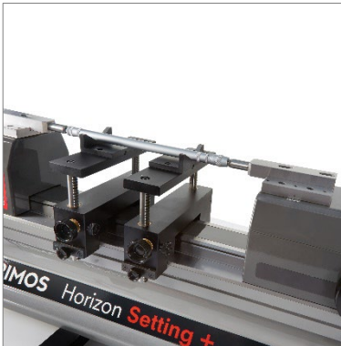
Setting of 2-point internal measuring equipment (TELMA7)
