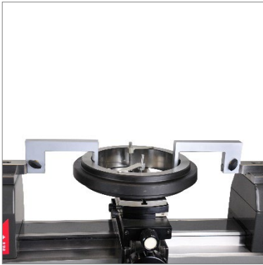
Checking of ring gauges (TA-SU-313, TA-MI-370, TA-SU-304)
