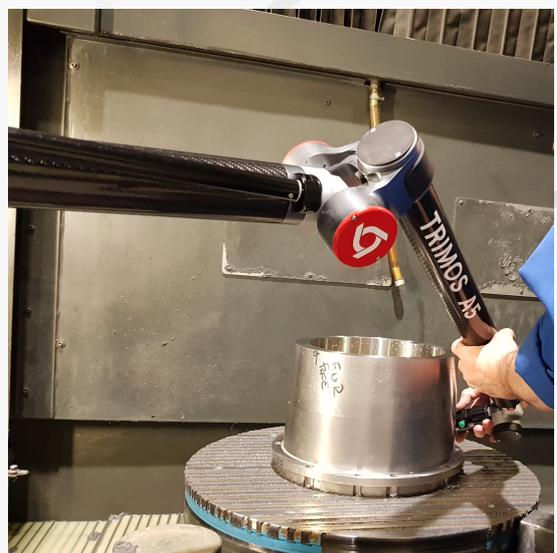
Additionally, the A5 can be equipped with a wireless Bluetooth device for complete portability, making it ideal for measuring large and heavy parts without moving them.
