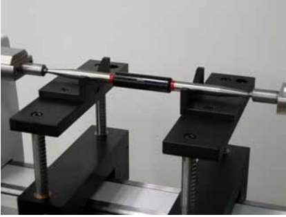
Checking of gauge bars
