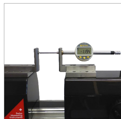
Checking of dial indicator (TEL5CN)
