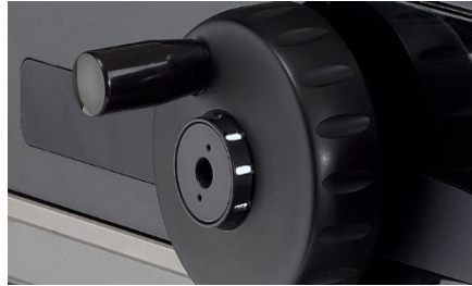
Setting force management with indicator
