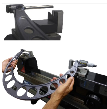
Manually checking of external micrometer (TEL5, TEL11)
